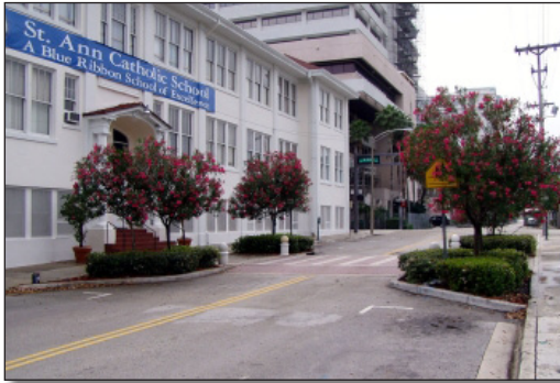
Example of a Mid-Block Bulb-Out
