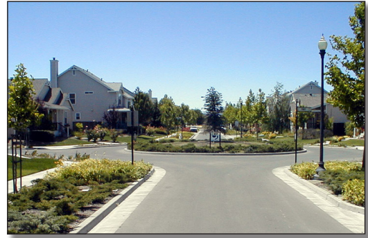
The Roundabout Above is Used to Control Traffic Speeds Entering a Neighborhood
